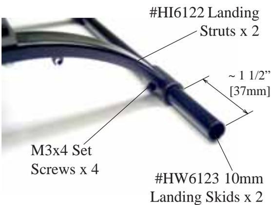
Assemble the landing skids onto the struts, note the correct direction is to have the struts sweep forward. Position the rear strut at approximately 37mm from the end and secure the skid with the M3 set screw. Leave the front loose for now.
