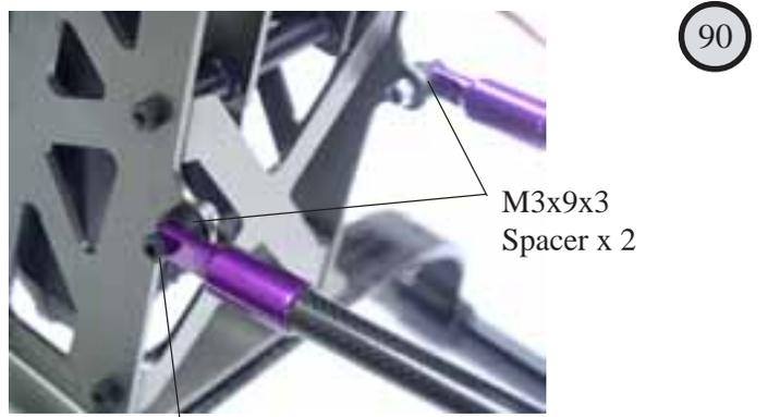
Attach the struts (aluminum or carbon) to the main mechanics using M3 socket screws, M3x9x3 plastic spacer on the outside and secure with M3 locknuts on the inside of the frames.
