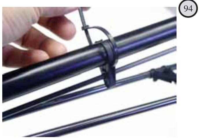
Remove the pushrod from the servo and slide through the entire range of movement. Continue adjusting the guides until the pushrod moves very smooth and then secure the tail guides with the cable ties.
