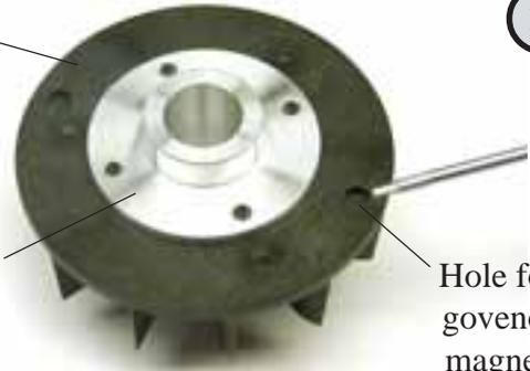
If a governor is planned to be installed, install the magnets into the holes already molded into the bottom of the cooling fan and attach the sensor mount, overlapping the engine bolts.
