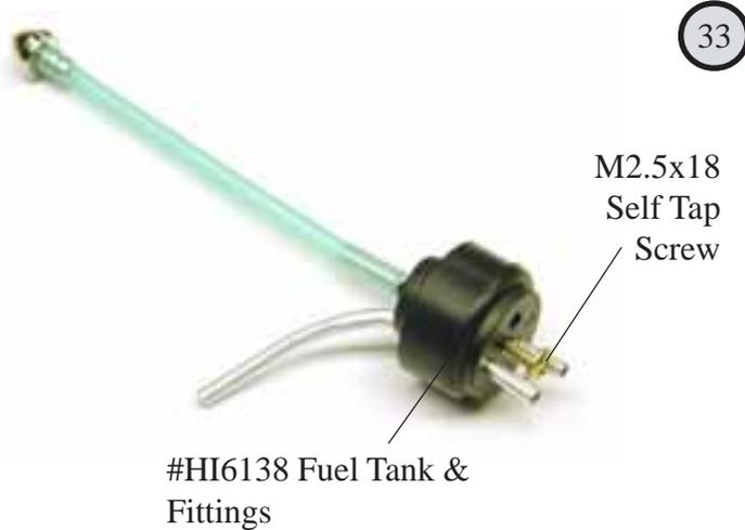
Assemble the fuel tank fittings. Gently bend the vent line and test until it reaches the top of the fuel tank. Order is larger outside cap, rubber stopper, smaller inside cap. Test the pickup line so the clunk stays at least 3/8" away from the wall.
