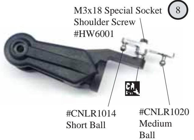
Attach the seesaw assembly with one M3x18 special socket screw threaded into the blade grip. Be careful not to over-tighten the screw.
