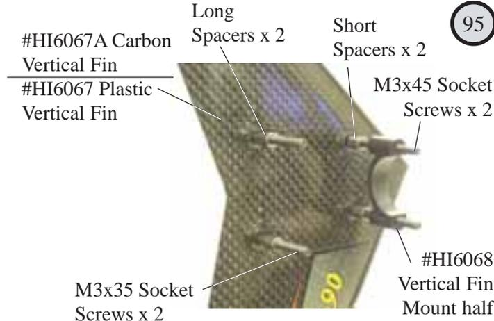
Insert the M3 socket screws through the holes in the carbon vertical fin. Slide the short spacers on the front bolts and the long on the rear bolts. Slide the vertical fin mount on after the short spacers.
