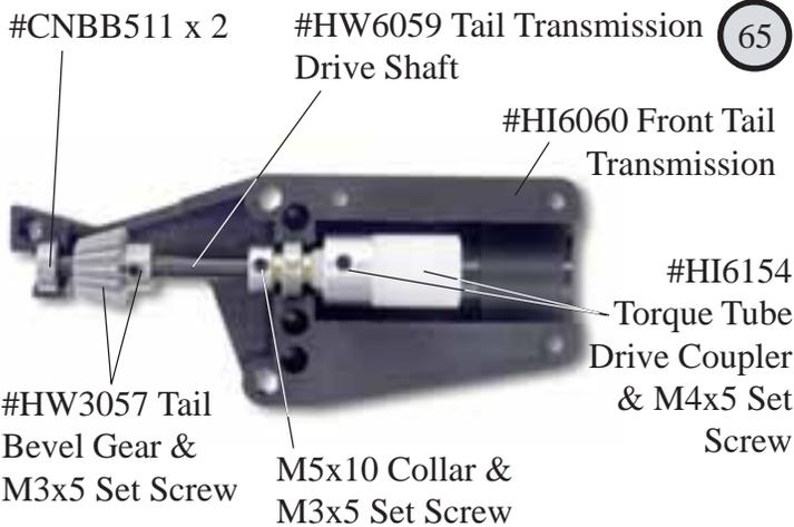
Insert the M3x5 set screw into the bevel gear and leave loose until the transmission is fitted to the mechanics. Set the gear mesh by running a single piece of paper between the bevel gear and the main gear. Once in position, locktite the set screw.
