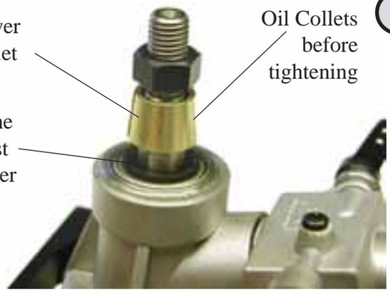
Ensure that the split in the collet is positioned away from slot for the Woodruff key. The lower collet is a tight fit to the crankshaft. Use the engine nut to start the collet onto the crankshaft, apply oil to collet.
