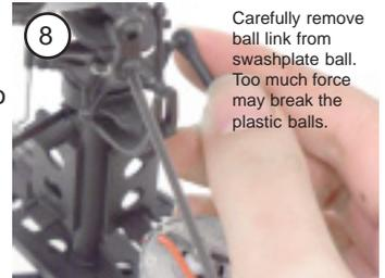
Carefully remove ball link from swashplate ball. Too much force may break the plastic balls.
