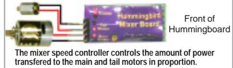
The mixer speed controller controls the amount of power transferred to the main and tail motors in proportion.
