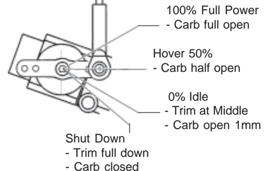
**Tip** If the Optional CN3059 Scale Muffler is going to be used, the stock plastic carburetor arm will not fit and the Optional CN2153 throttle extension needs to be used.
