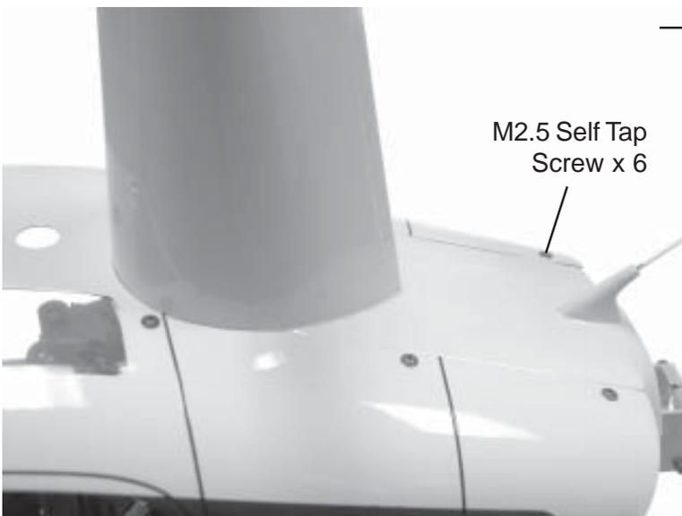
**STEP 54 Front Landing Gear Mounts**
