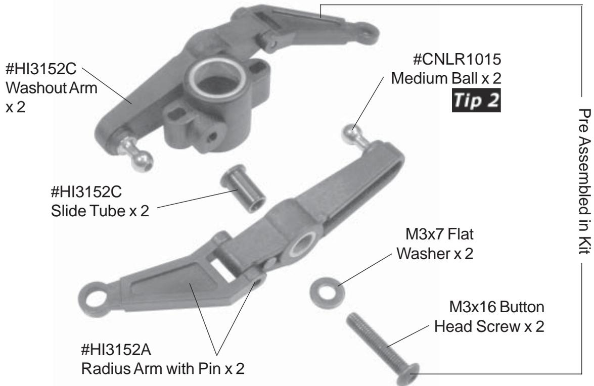
**Step 8 CCPM (cyclic collective pitch mixing) Swashplate Assembly**
