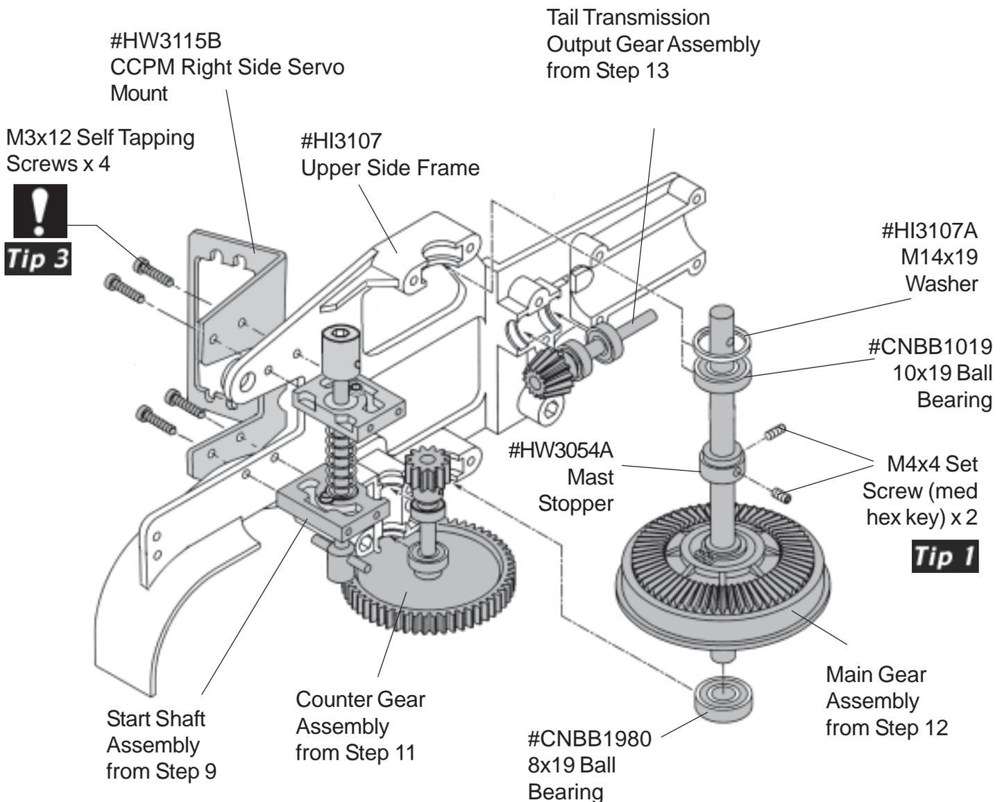
**Note 1:** Be careful when tightening the eight 3x12mm self tapping screws into the start shaft block assemblies as excessive force will strip out the plastic holes.
