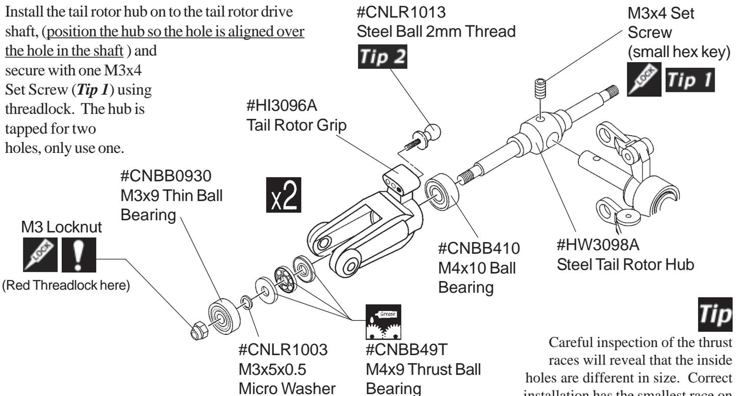
Install one short steel ball into the upper right hole in the tail rotor grip (**Tip 2**).
