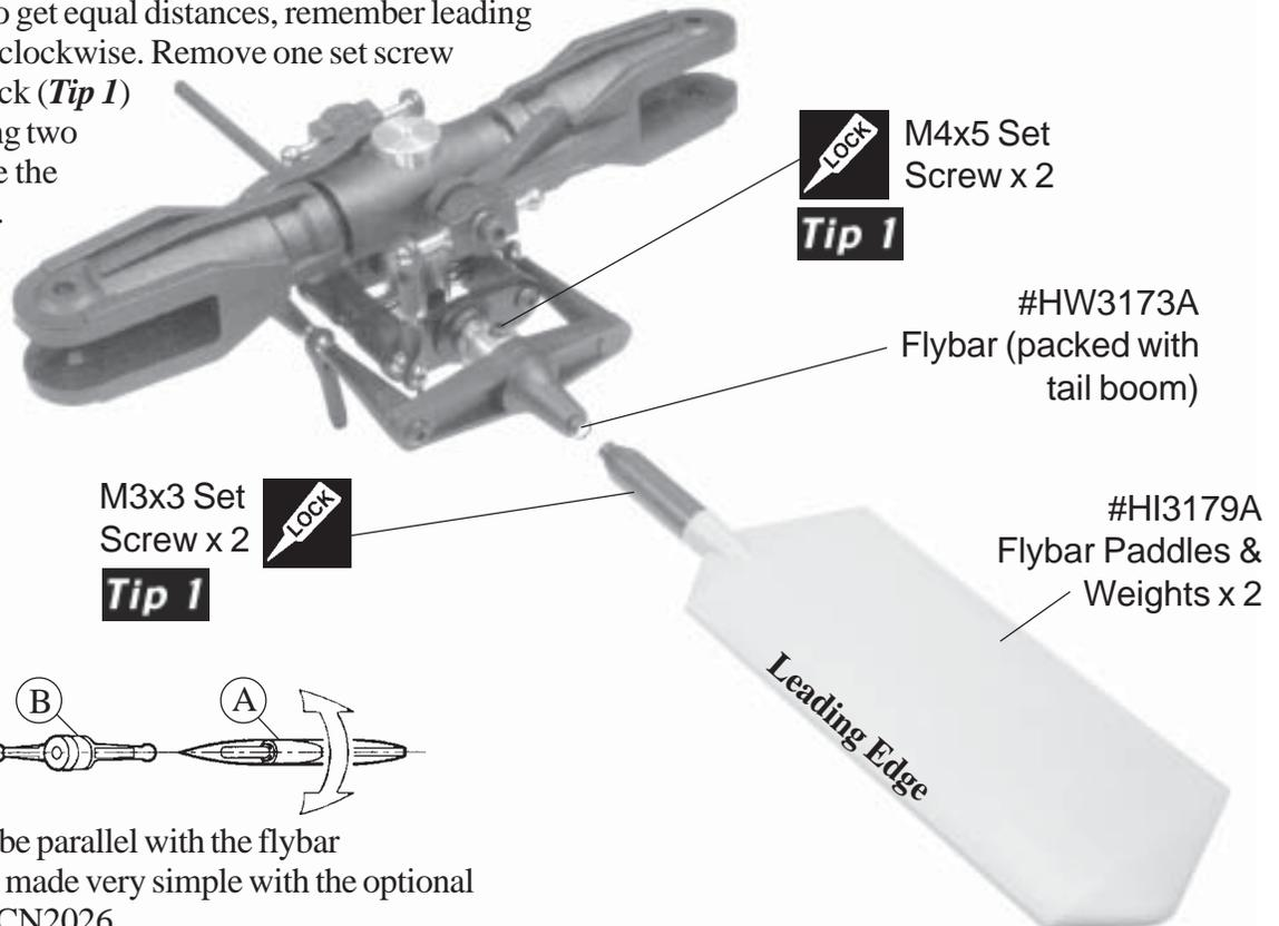
Align each paddle 'A' to be parallel with the flybar control arms 'B'. This is made very simple with the optional pitch and paddle gauge CN2026
