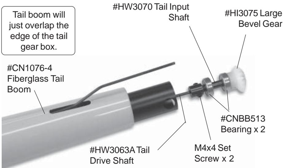
**Tip:** Before assembling the tail gear box, verify that the tail input shaft rotates straight on the end of the tail drive shaft by rotating slowly in your fingers. If the tail input shaft does not turn true, adjust the tension of the M4x4 Set Screws. The problem is a result of the set screws not having the same tension.
