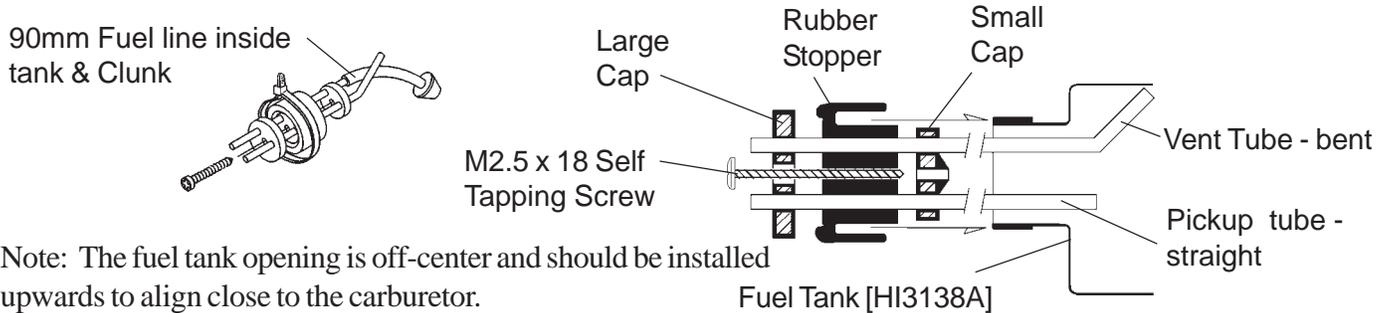
Note: The fuel tank opening is off-center and should be installed upwards to align close to the carburetor.
