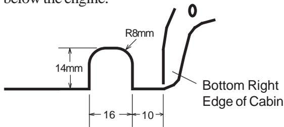
The left side of the fiberglass cabin needs to be ground out for the exhaust pipe to clear the body. We have listed a hole size that is larger than the tube as we also suggest that an exhaust deflector is used to keep the gases away from the inside of the cabin.
