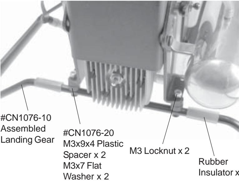
**STEP 55 Rear Landing Gear Mounts**
